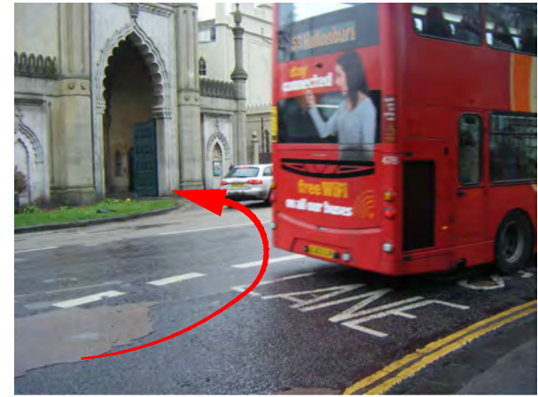
Risk of congestion and blocking movements as larger vehicles swing wide to enter.
