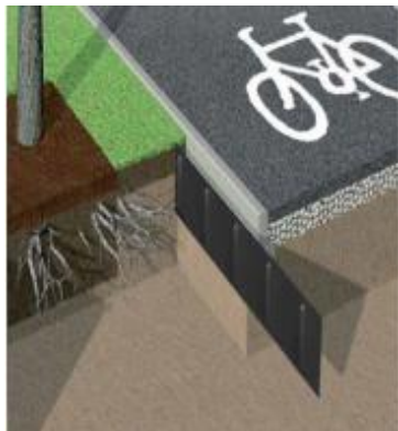
Image 1: identifying tree root barriers to be used within grass verges
