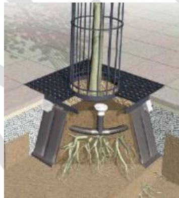
Image 2: identifying tree root deflectors to alleviate root damage within hard surfaces.
