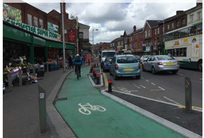
Figure 1.10: Example of kerb-segregated cycle track
