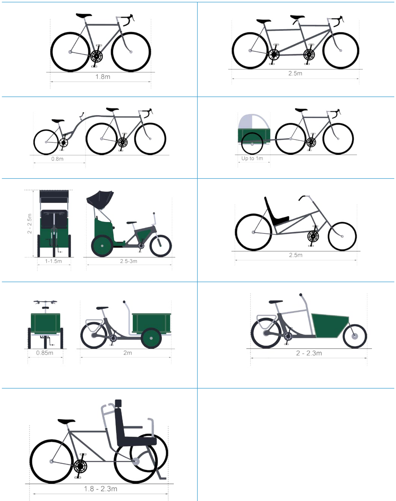
Figure 5.2: Typical dimensions of cycles
