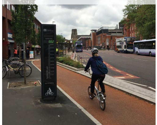
Figure 11.16: Real time cycle counter in Manchester
