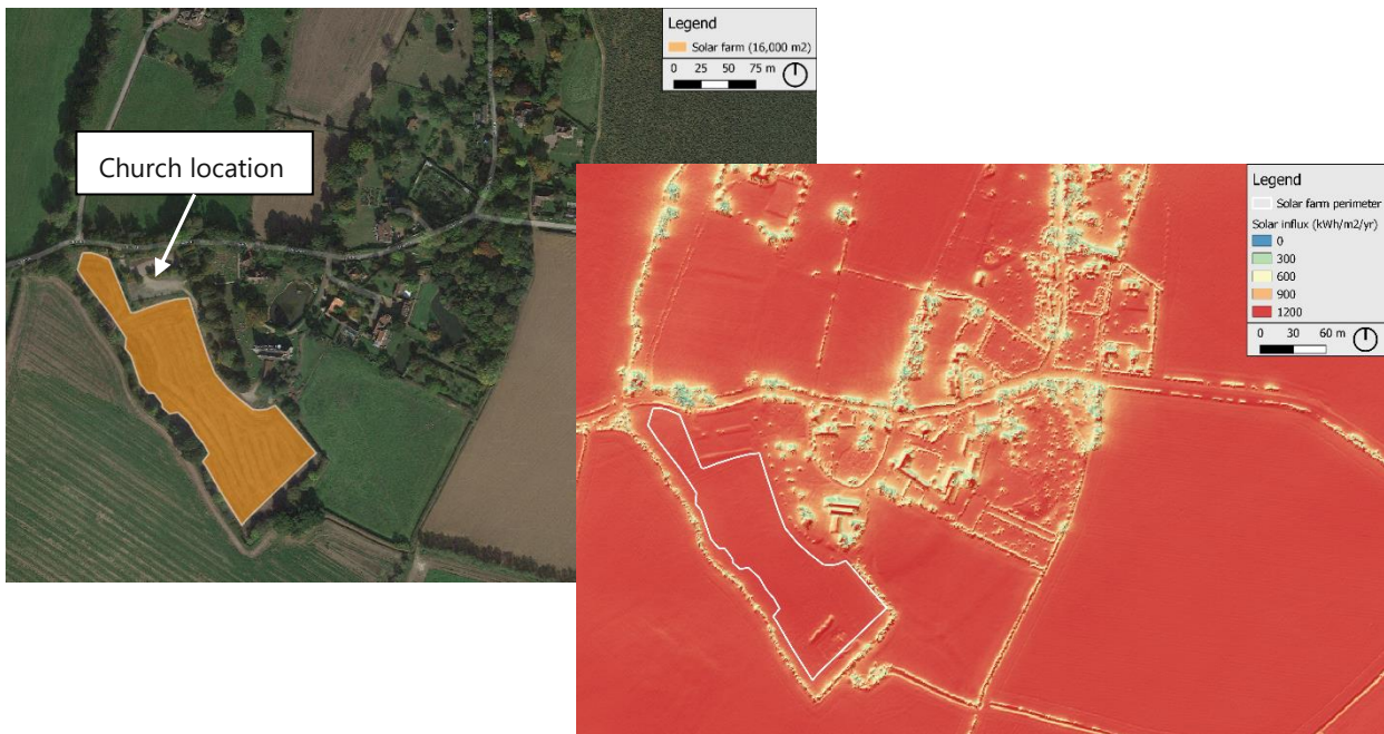
Figure 8—7 Proposed solar farm site for Barcombe Church and solar energy data. Modelling of solar resource is carried out in QGIS using the UMEP SEBE tool, with meteorological data from PV-GIS.
