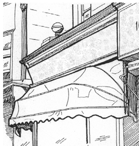
An unacceptable fixed Dutch blind x
